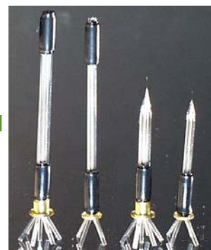
Unpulled and Pulled 7, 4-barrel Pipettes
