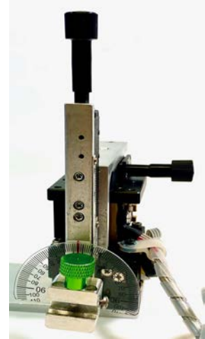
Right side 3D Micromanipulator with coarse 2D adjustment
