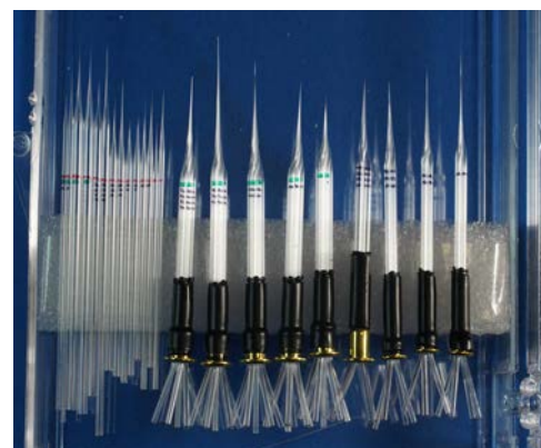
Pulled Single, 3, 4, 7- barrel Pipette Samples for Every Shipped Out Unit
