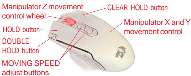
Wireless Mouse for left side (Holding) control
