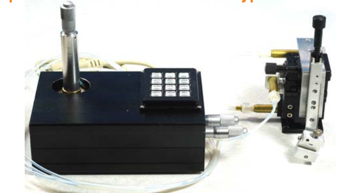
JHM-3L-PM1 3D Hydraulic Joystick Micromanipulator with PM-1000 Remote Keypad
