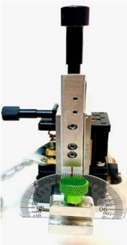
Left side 3D Micromanipulator with coarse 2D adjustment
