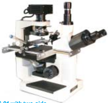
IMS-01 with two-side micromanipulator mounting adaptors
